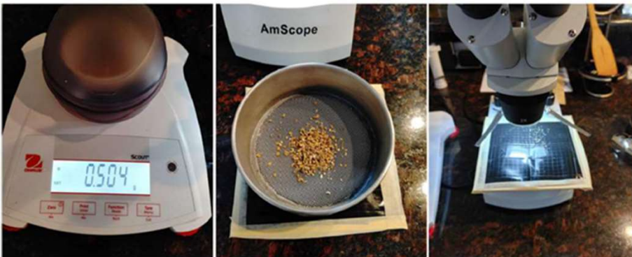
Microbalance, sieve method and sticky counting board
